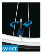
Tighten the new valve. For tubeless installations ensure valve rim nut remains tight.
